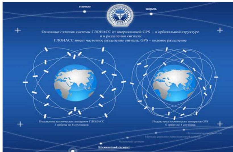
Figure-1: shows the orbit and constellation of GLONASS (left) and GPS (right).
